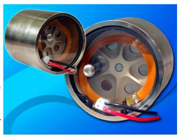
connector. The moving coil and termination is simply plugged in via any length of tail. This makes the device neater and because the flex is terminated directly onto the coil, less stress is created at the joint making it resistant to damage or disconnection through constant movement and material stress.
